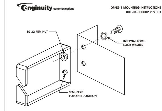
D-RING IS INSTALLED INTO THE TWO HOLES NEAREST THE BEND ON THE MOUNTING BRACKETS IN EITHER THE 19" OR 23" CONFIGURATION. THE SCREW INSTALLS FROM THE BACK SIDE OF THE BRACKET INTO THE PEM NUT IN THE D-RING.
