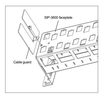
Figure 1. Cable guard attachment to SIP-3600.
