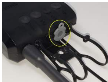
Cleaning Adapter Positioned in Fiber Terminal Port
